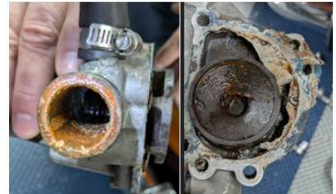
Water pump shows rust and rust scum on the impeller. The scum at the upper right of the impeller is liquid gasket material from a prior install process years ago.
