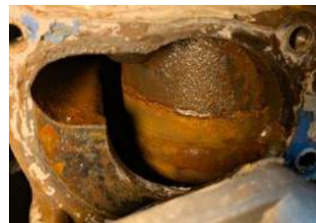
Behind water pump looking at cylinder 1 casing
