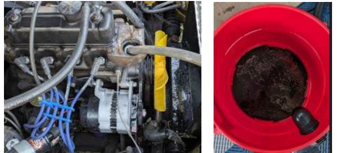
Left: Garden hose flushing of the engine block. Right: Here is the extracted EvapoRust, came out black.
