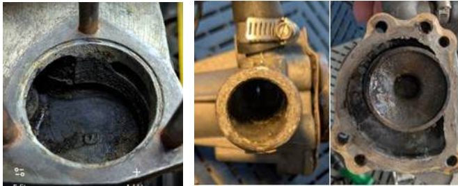
Left: Thermostat bay after: looks much better!" Right: Water pump after—I did replace the pump anyway with a new one that had come with the car purchase
