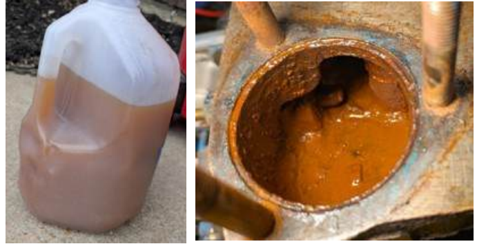
Left: This was originally new yellow coolant, three months prior. Right: Removing the thermostat really explained my problem.
